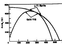
Fig. 1 Saturation magnetization versus temperature of 600 G LiTi ferrite and GdAlYIG.
